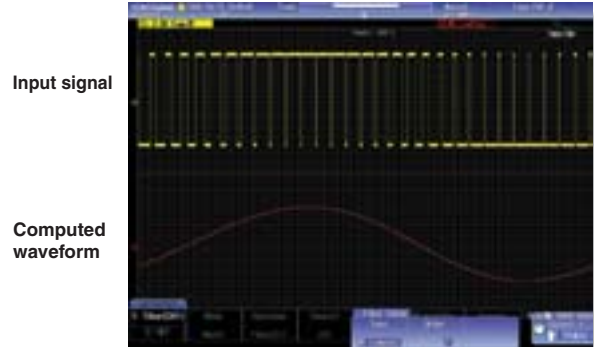
Filtering of a PWM waveform using computation
