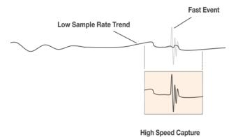
As an example, it is possible to set waveform triggers and capture 5000 high-speed transient events at 100 MS/s while at the same time continuously recording a trend measurement at 10 kS/s for 10 hours.
