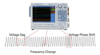
A ScopeCorder is sometimes referred to as "the ultimate trigger machine", and is packed with basic and enhanced triggers. A feature called "action on trigger" allows the user to leave a ScopeCorder unattended and automatically save the waveform to a file or send an email for notification of a trigger event.
