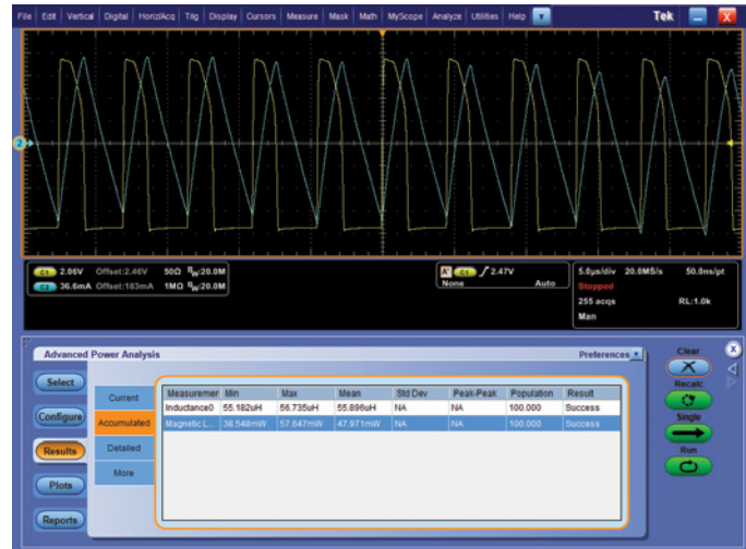
Figure 20. Inductance and magnetic loss measurements.
