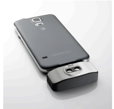
Figure 22.3 2015: FLIR One, an accessory to iPhone and Android mobile phones. Weight: 90 g (3.2 oz.).
