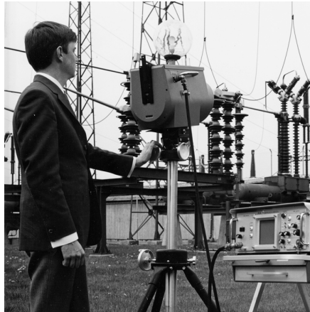
Figure 22.2 1969: Thermovision Model 661. The camera weighed approximately 25 kg (55 lb.), the oscilloscope 20 kg (44 lb.), and the tripod 15 kg (33 lb.). The operator also needed a 220 VAC generator set, and a 10 L (2.6 US gallon) jar with liquid nitrogen. To the left of the oscilloscope the Polaroid attachment (6 kg/13 lb.) can be seen.
