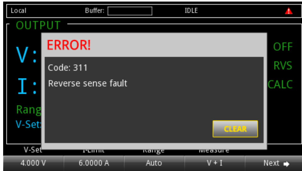
Figure 47: Reversed sense leads error
