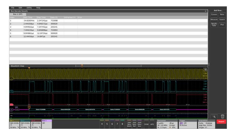
Consider an example system with daisy-chained SPI architecture. This subsystem controls a voltage-controlled oscillator (VCO) that provides the RF clock to the rest of the system. The VCO is initialized by the main CPU by writing six 24-bit words to the VCO. The signals appear to meet the electrical specifications for SPI, but the VCO is not generating the right frequency.
