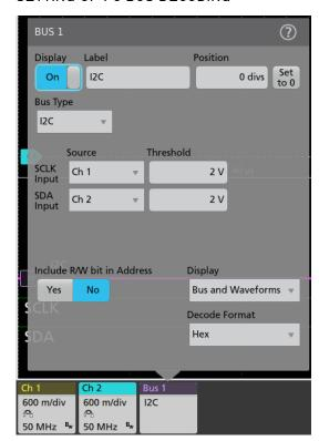
On Tektronix oscilloscopes, pressing the front panel Bus button enables you to define inputs to the scope as a bus. By simply defining which channels clock and data are on, along with the digital threshold levels used to determine logic ones and zeroes, you enable the oscilloscope to understand the protocol being transmitted across the bus.
