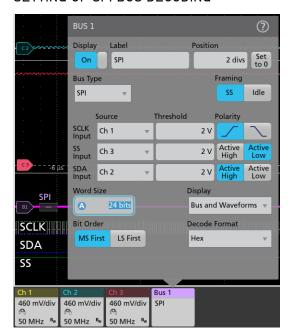
In this example, the SPI signals are being captured using passive probes on the analog channels (channel 1, channel 2 and channel 3) on the oscilloscope. Digital channels can also be used for bus decoding. Using the Bus configuration menu, you can define an SPI bus by specifying which channels are connected to the clock, data, and slave select signals, the thresholds, polarities, and word size.
