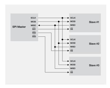
Rather than having unique addresses for each device on the bus, SPI uses the SS line to specify which device data is being transferred to or from. As such, each unique device on the bus needs its own SS signal from the master. If there are 3 slave devices, there are 3 SS signals from the master, one to each slave.
