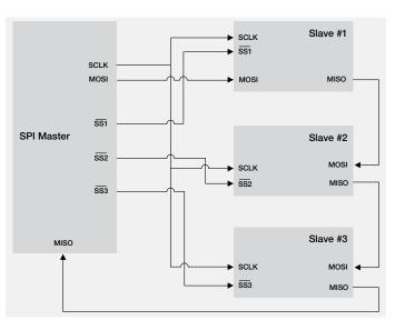
SPI can also be wired with the slave devices daisychained, each performing an operation in turn, and then sending the results back to the master (which can be used to verify the integrity of the data path). In some cases, where communication from the slave back to the master is not required, the MISO signal may be left out altogether. In other cases there is only one master and one slave device and the SS signal is tied to ground. This is commonly referred to as 2-wire SPI.
