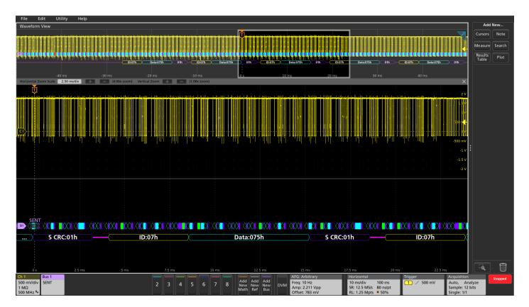
The decoded SENT bus can display both fast and slow channel packets in a single waveform display, with the slow channel packets shown below the fast channel packets.
