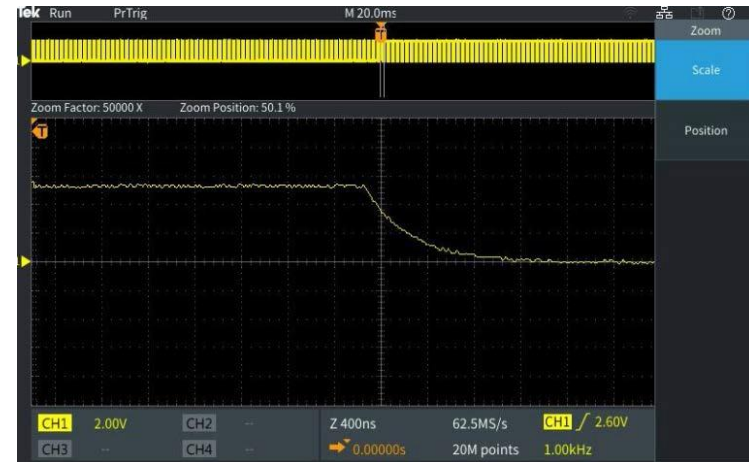
Figure 9. Zooming in on a falling edge
