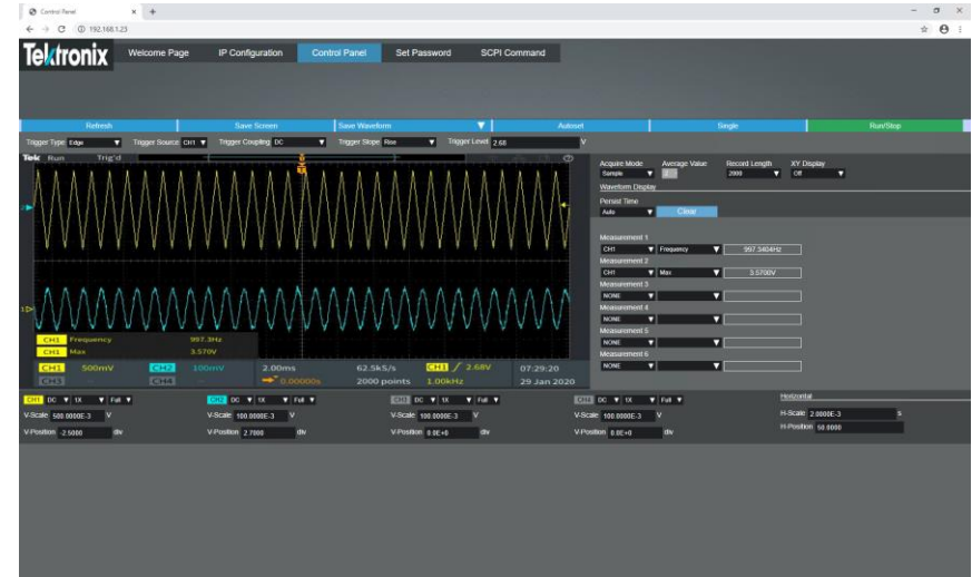
Figure 22. On the PC, the IP has been entered into the address box of the browser, and autoset has been performed remotely
