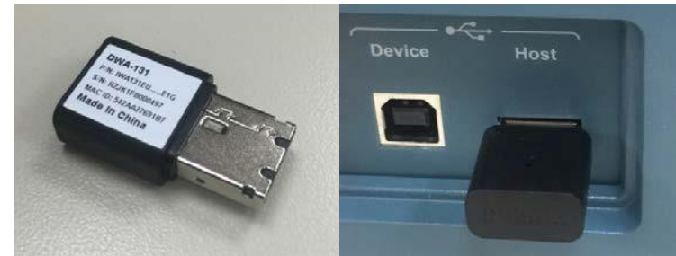
Figure 19. Insert the TEK-USB-WIFI adapter to enable wireless communications
