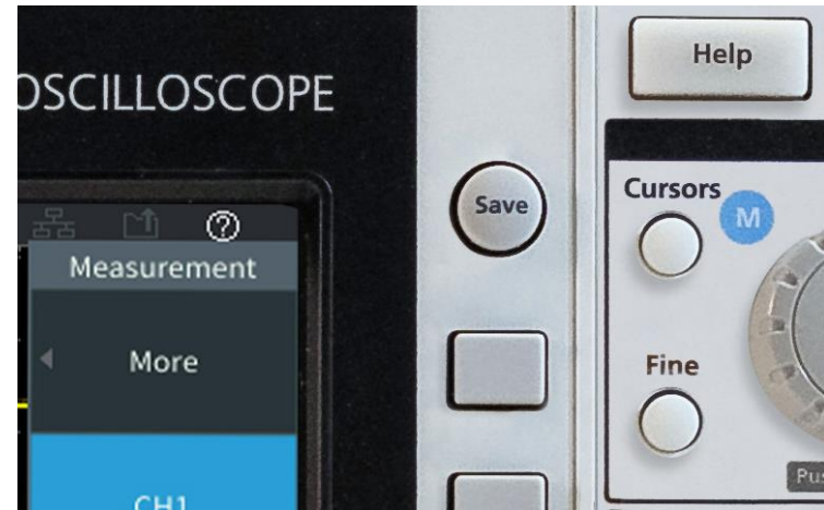
Figure 17. One Touch Save button quickly lets the user capture information from the instrument.
