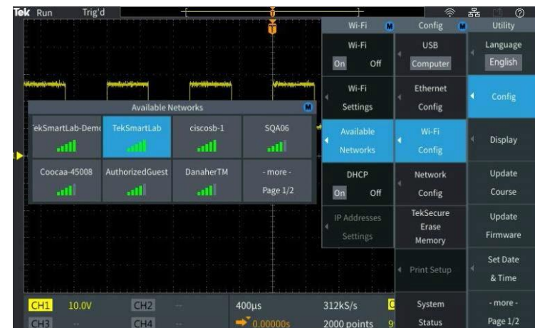
Figure 20. Configuring Wi-Fi communications via the Utility Menus
