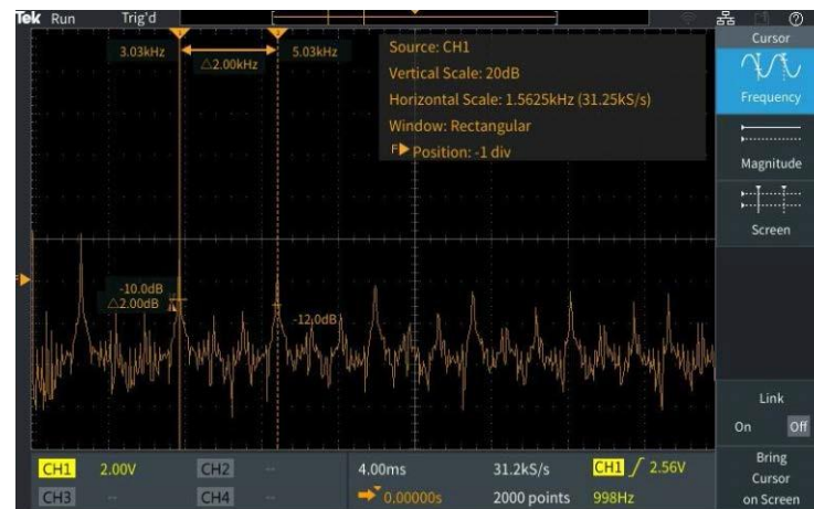
Figure 15. Cursors positioned on the 3 kHz and 5 kHz harmonics of the 1 kHz probe comp output .
