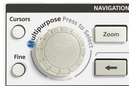
Figure 10. Location of the Cursors and Fine buttons (two-channel model shown)
