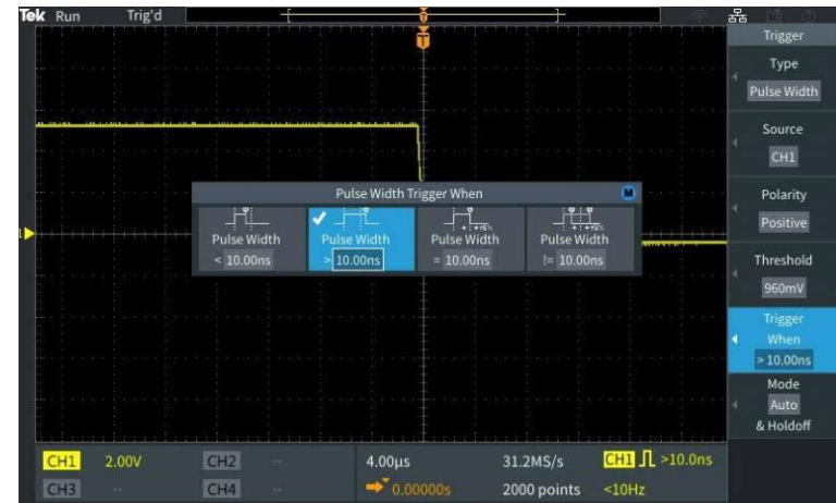
Figure 7. Setting pulse width trigger parameters
