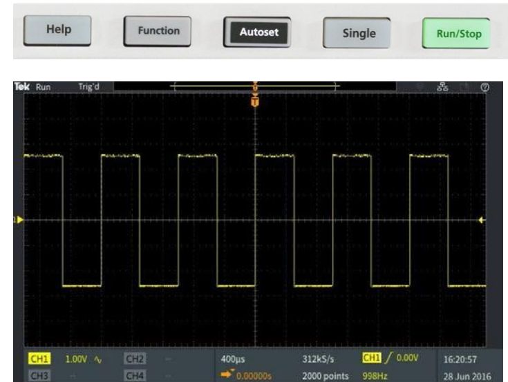
Figure 5. Autoset button and display after pressing autoset
