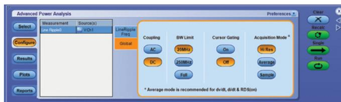
Figure 18. Line Ripple configuration tab for DPOPWR.
