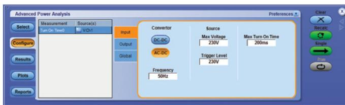
Figure 22. Turn-on time configuration tab for DPOPWR.
