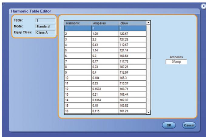
Figure 25. Pre-Compliance Testing results table using DPOPOWER.
