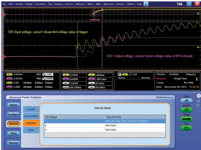
Figure 23. Turn-on Time results using DPOPWR.
