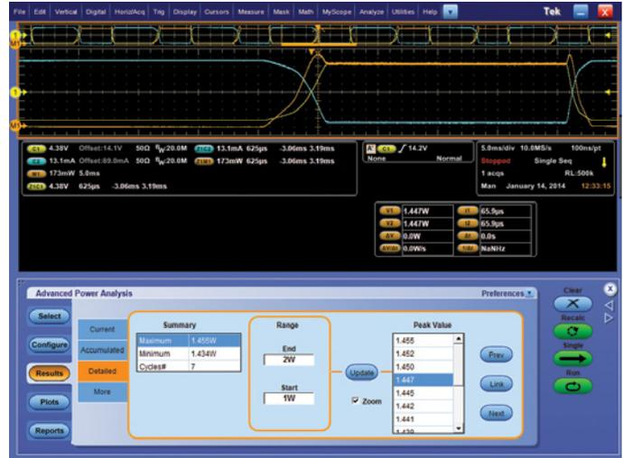
Figure 10. Switch Finder results tab displaying energy loss.
