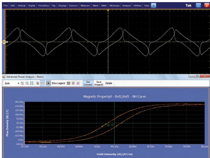
Figure 4. Magnetic Characteristics display using DPOWR.
