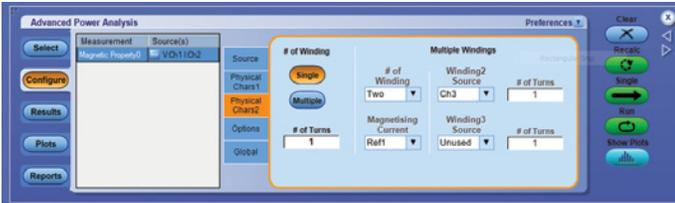
Figure 6. DPOPWR configure tab for B-H Plots.
