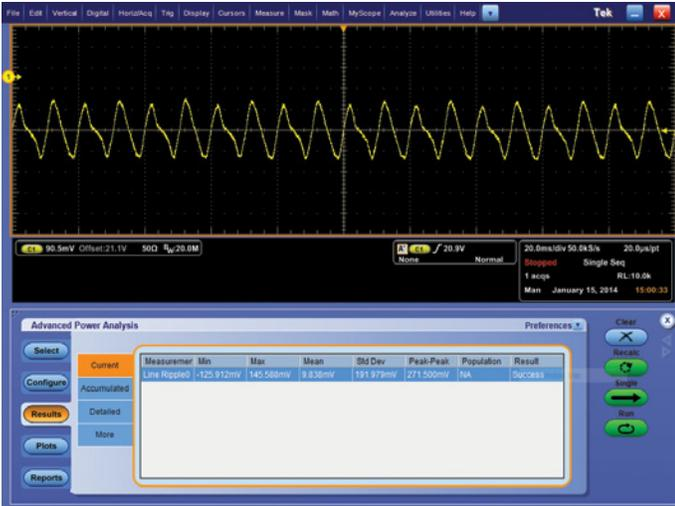
Figure 19. Switching Ripple results using DPOPWR.
