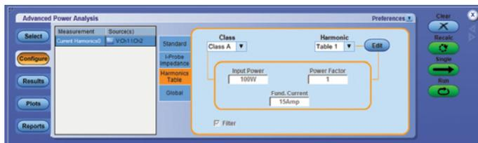
Figure 24. Pre-Compliance Testing configuration tab on DPOPOWER.
