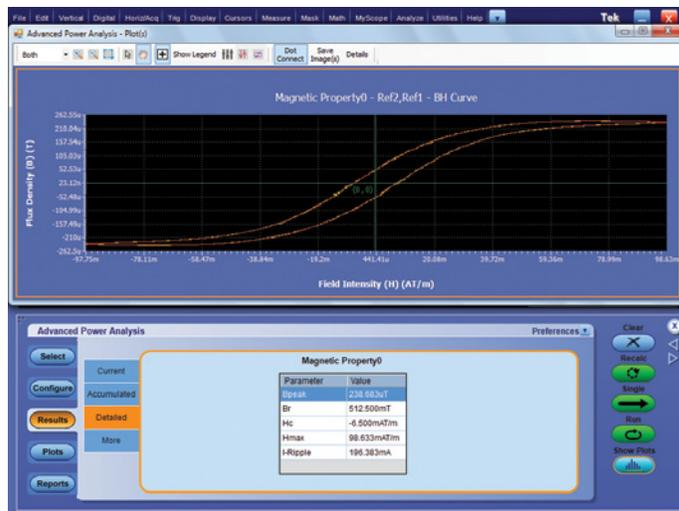
Figure 5. Magnetic Power Loss results using DPOWR.
