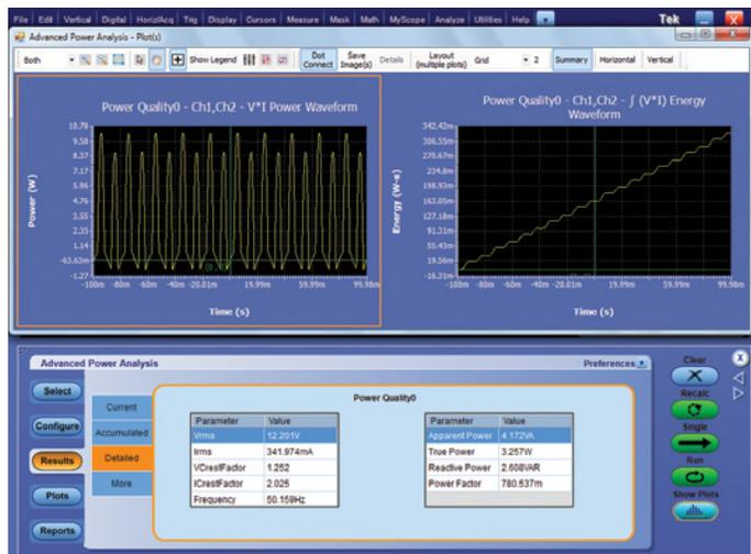
Figure 14. Power Quality results using DPOPWR.
