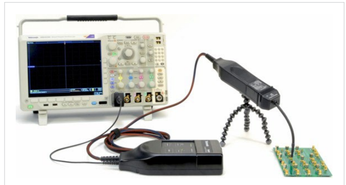
Using a Tektronix oscilloscope and IsoVu probe, Panasonic was able to significantly reduce the time required for analysis of the halfbridge circuit and the signal.
