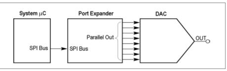
Figure 50. Mixed signal chain block diagram.
