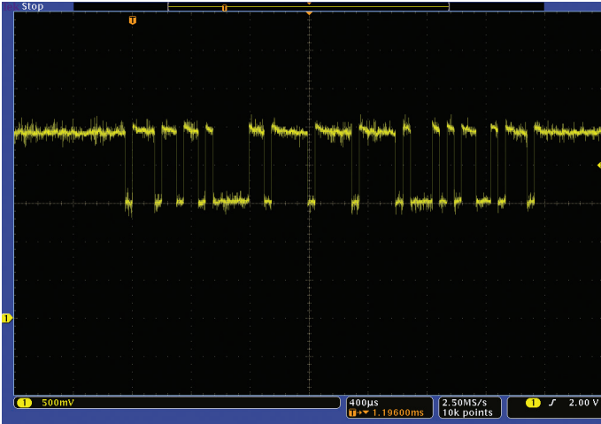
Figure 2. One message acquired from a CAN bus.
