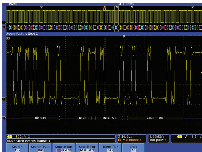
Figure 44. Searching on specified identifier and Data in a CAN bus acquisition.
