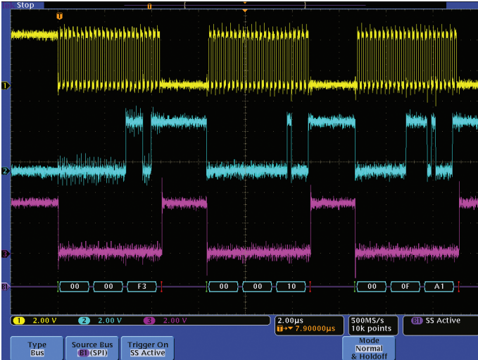
Figure 13. Correct synthesizer configuration messages.
