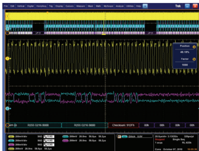
Figure 53. MSO70000C analog-channel decoded display of a Packed Pixel Stream, showing a checksum error.
