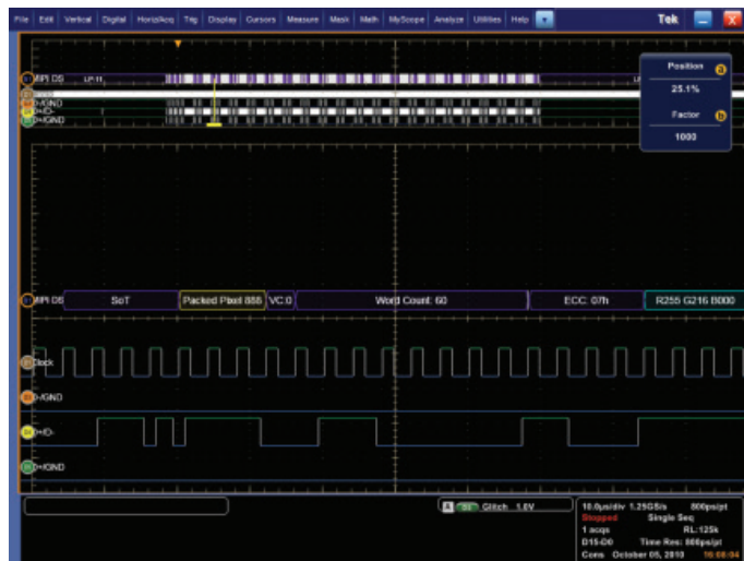
Figure 52. MSO70000C digital-channel decoded display of a Packed Pixel Stream, 24-bit RGB 8-8-8 Format long packet.
