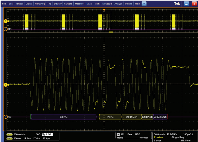
Figure 23. Decoded High-speed USB 2.0 waveform captured with serial triggering on an MSO5204 with option SR-USB.
