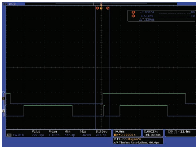
Figure 13. Triggering on 727.3 ps glitch on the bottom LVPECL signal.
