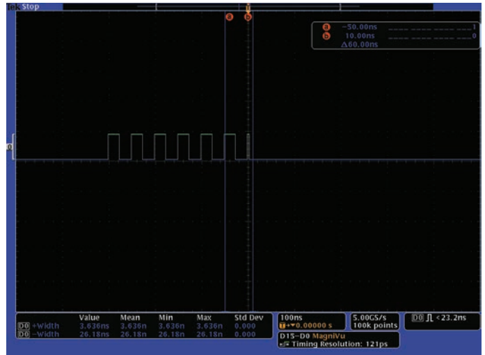
Figure 11. Triggering on positive pulse width error of 3.636 ns.
