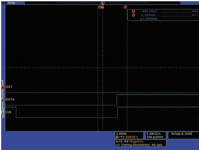
Figure 22. Triggering on the D-Flip-Flop data changing in the setup/hold window between cursor 'a' and 'b' around the rising clock edge.
