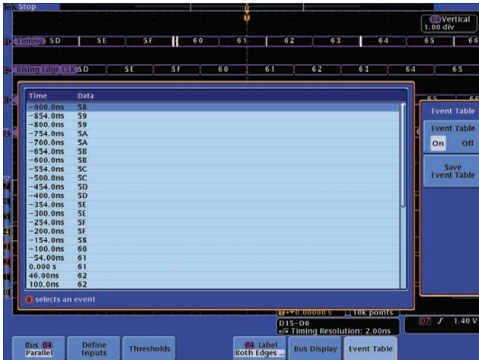
Figure 3. Decoded data is shown in an event table which is similar to a logic analyzer's state acquisition display.
