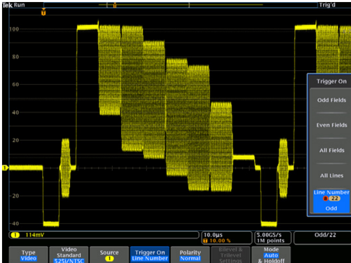
Figure 6. The 4000 Series' video trigger allows convenient selection of video standard, source, component to trigger on, polarity, and holdoff settings. In this example, the oscilloscope has triggered on line 39 of the Odd Field of an NTSC signal.
