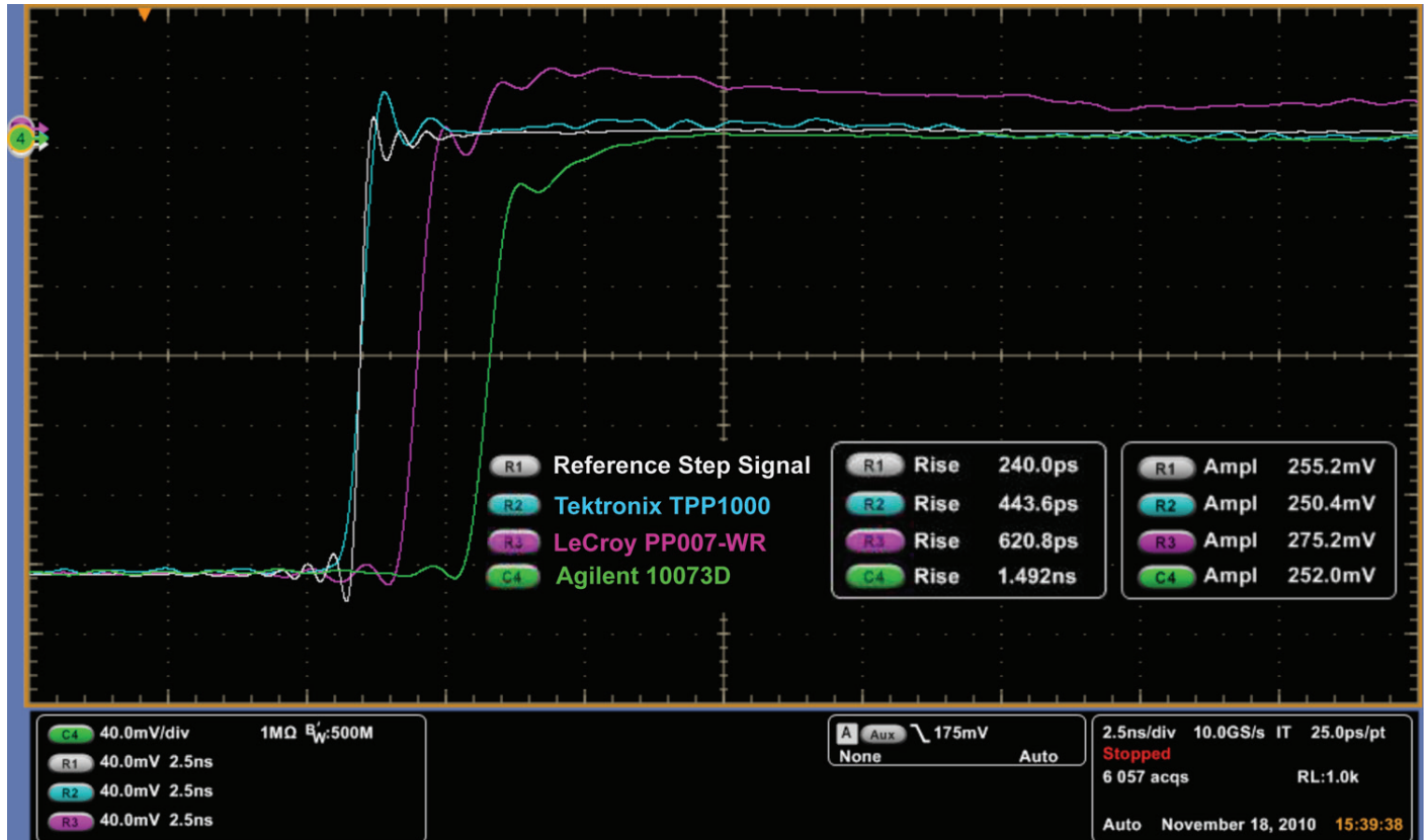
Figure 1. Rise Times of Tektronix, LeCroy, and Agilent Standard Passive Voltage Probes.
