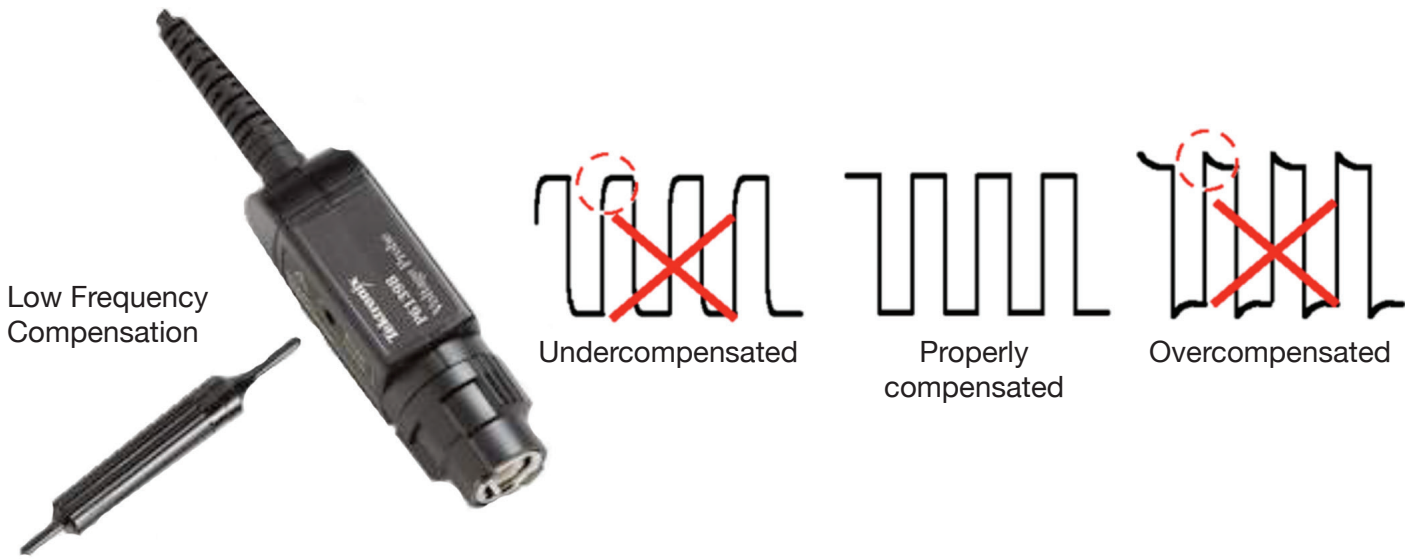
Figure 4. Low Frequency Probe Compensation.
