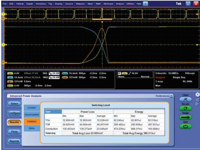
Figure 5. DPOPWR automated switching loss measurement.
