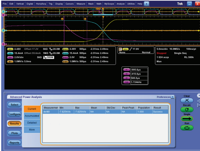
Figure 7. Automated slew rate measurement on MOSFET gate.
