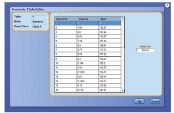
Figure 25. Pre-Compliance Testing results table using DPOPWR.
