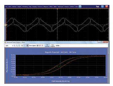
Figure 4. Magnetic Characteristics display using DPOPWR.
