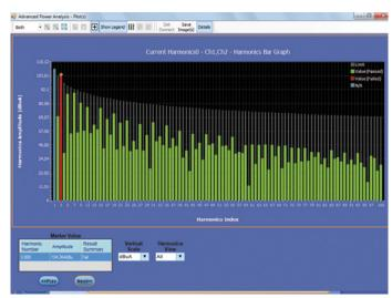
Figure 16b. Up to 100 Current Harmonics are displayed in graphical form using DPOPWR.
