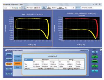
Figure 8. Switching Loss Measurements Using DPOPWR.
