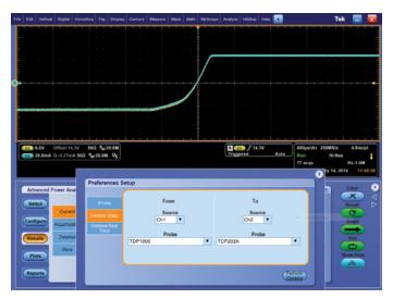
Figure 2. Static Skew Compensation Between Two Probes, AFTER Adjustment.
