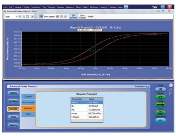
Figure 7. B-H Plot using DPOPWR.
