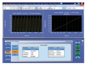
Figure 14. Power Quality results using DPOPWR.
