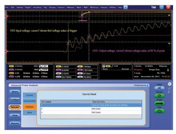
Figure 23. Turn-on Time results using DPOPWR.
