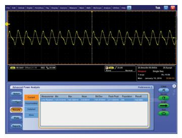
Figure 19. Switching Ripple results using DPOPWR.
