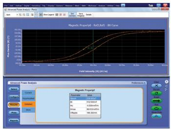
Figure 5. Magnetic Power Loss results using DPOPWR.
