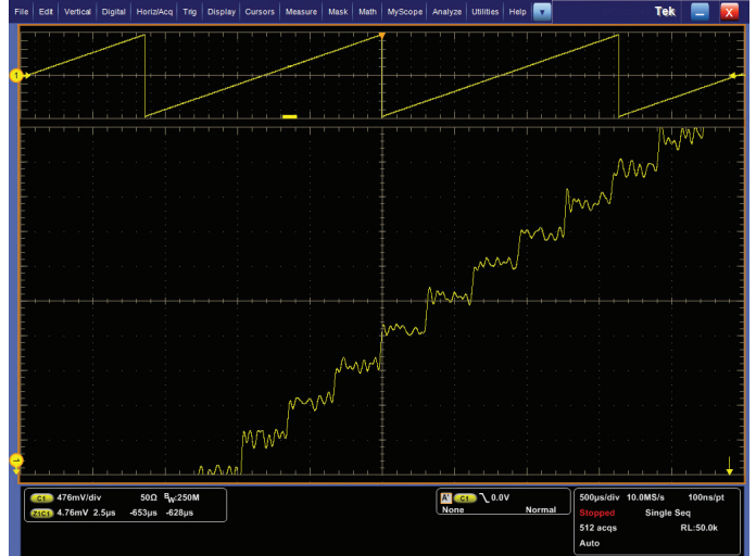
Figure 21. Zoomed display of the same high-resolution ramp signal, based on a large number of averages, showing significantly higher vertical resolution.
