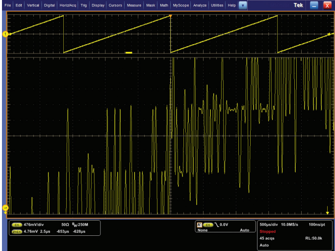
Figure 20. Zoomed display of a high-resolution digital ramp signal, showing digitizing noise due to limited resolution in the 8-bit ADC.
