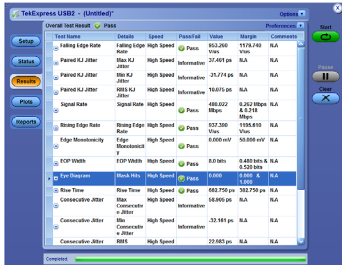
Figure 2. Measurement results are automatically displayed using the TekExpress USB2 compliance test package.
