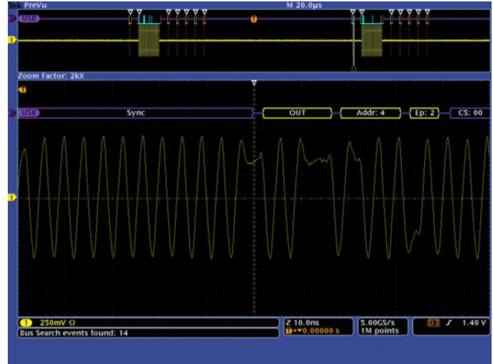
Figure 17. Simplified display, showing only the differential high-speed USB analog signal and the decoded bus.
