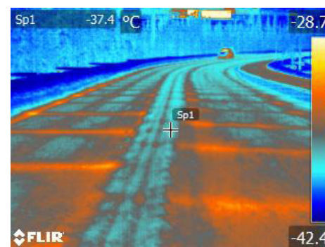
Thermal imaging can be used to see whether cooling devices of road infrastructures are working effectively.
