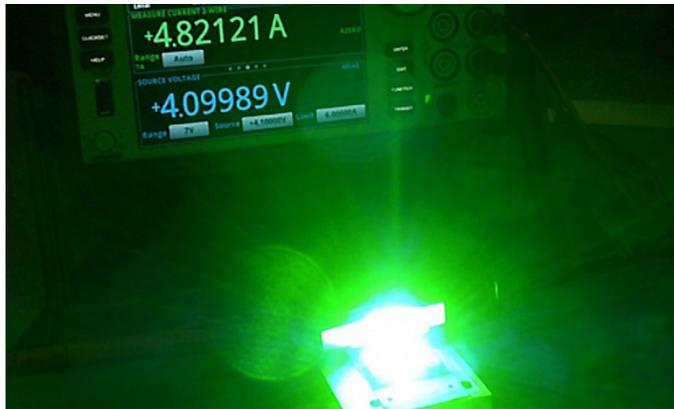
FIGURE 13: HBLED illuminated at 4.1 volts and 4.8 amps.
