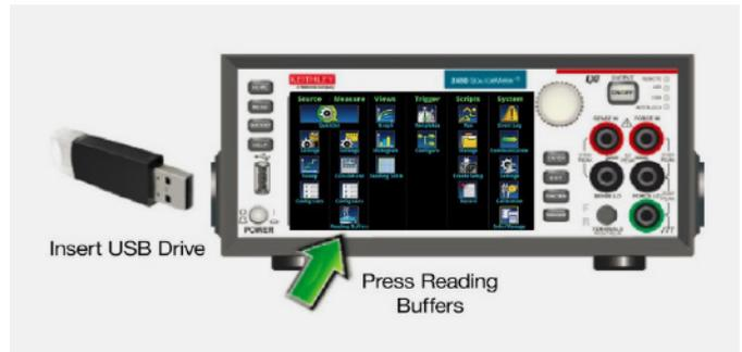
FIGURE 14: Saving data to a USB drive.
