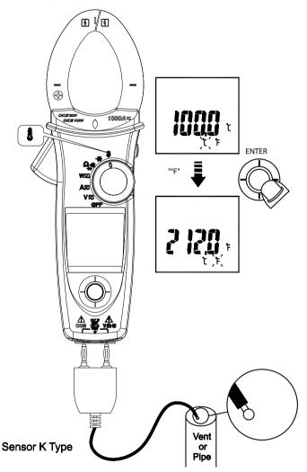
Don't take any high voltage measurement prior to accurate  $^\circ C^\circ F$  measurements.
