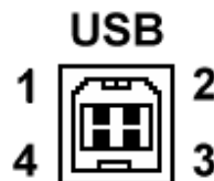
Figure 3-2: USB Connector pin orientation
