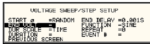
Figure 3-19: VOLTAGE SWEEP/STEP SETUP screen
