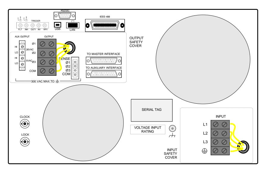
Figure 3-1: Rear Panel Connector Locations – Lx Series
