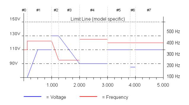
Figure 4-12: Sample Transient Output Sequence
