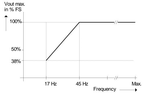
Figure 2-7: Voltage / Frequency Rating.
