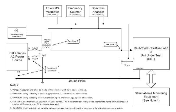
Figure 11-10: Required SVF-106 Test Setup.
