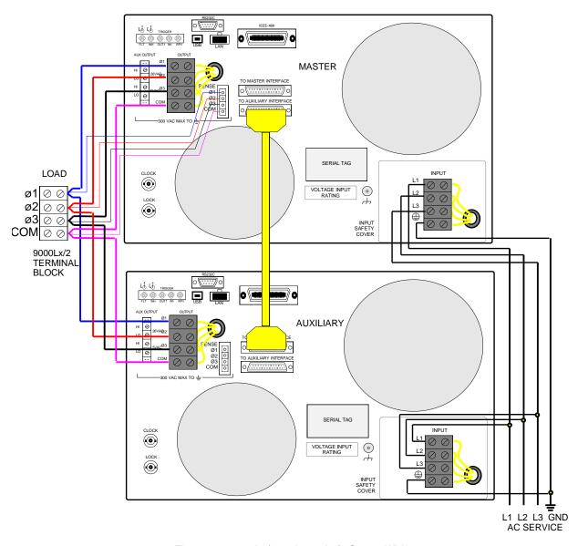
Figure 3-3: 9000Lx/2 and 9000Ls/2 Output Wiring
