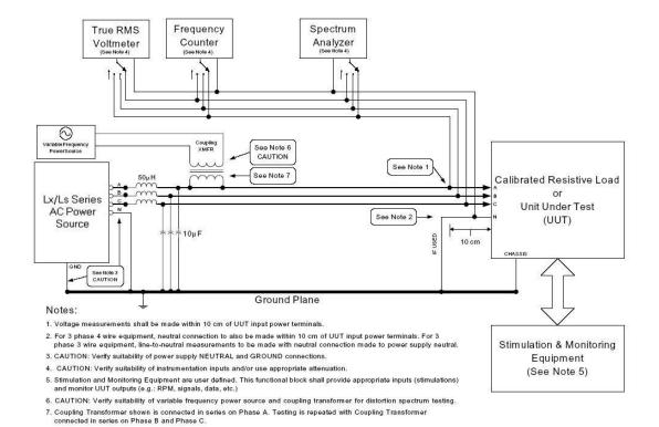
Figure 11-11: Required TVF-106 Test Setup.
