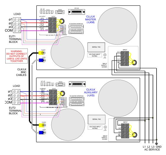
Figure 3-7: Clock and Lock Connections
