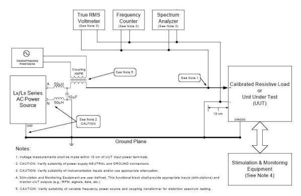
Figure 11-8: Required SAC-106 Test Setup.
