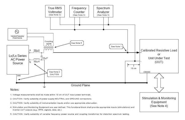
Figure 11-12: Required SXF-106 Test Setup.
