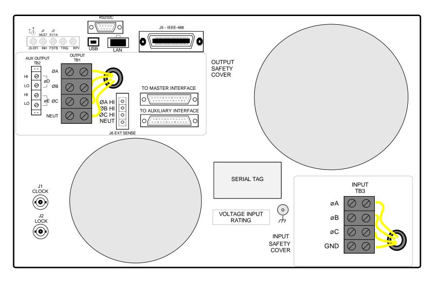
Figure 3-2: Rear Panel Connector Locations – Ls Series
