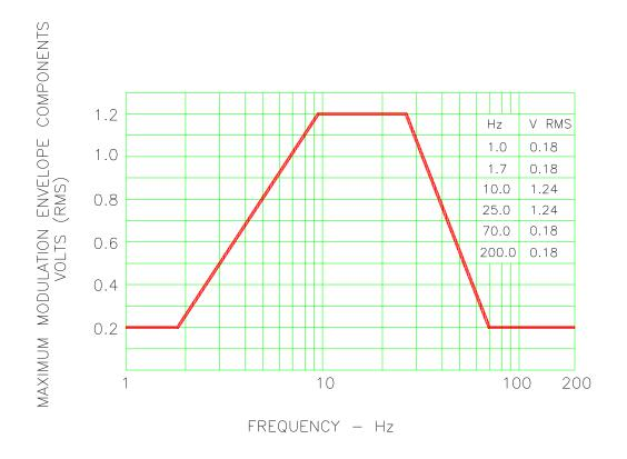
Figure 8-4: Voltage Modulation - Frequency characteristics
