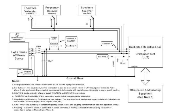
Figure 11-9: Required TAC-106 Test Setup.
