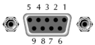
The plug pins of RS232
