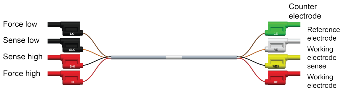
Figure 5: Cable assembly connector labels and definitions
