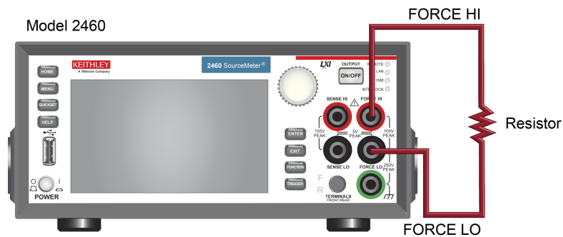
Figure 19: Model 2460 2-wire front-panel connections
