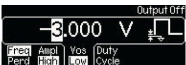
Figure 5-2: Setting the low-voltage level
