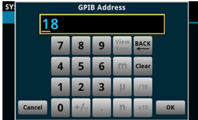
Figure 2: Front-panel keyboard for GPIB Address entry
