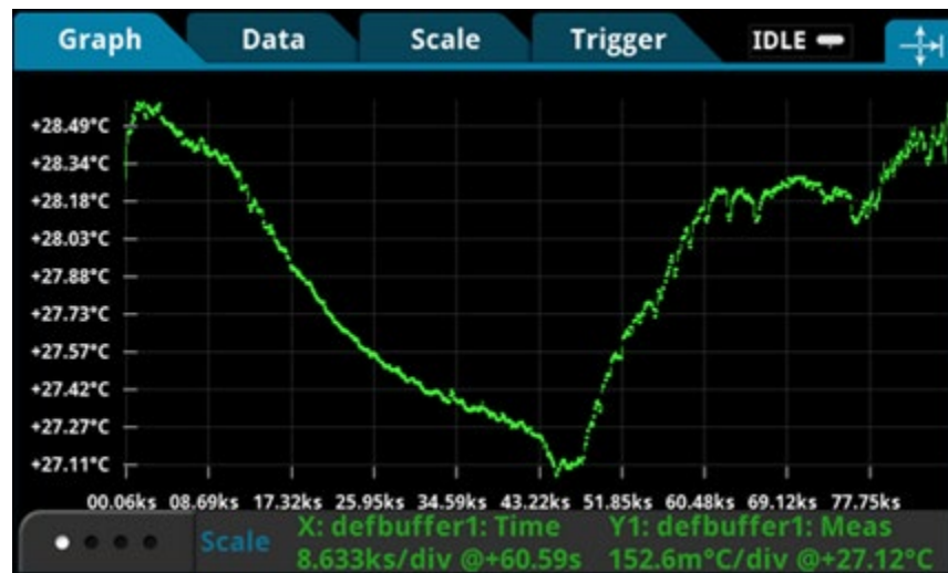
Figure 30: Model DMM7510 graph of temperature measurements
