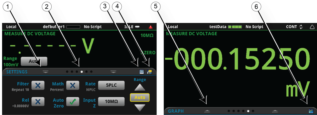
Figure 4: Model DMM7510 swipe screens, maximized and minimized
