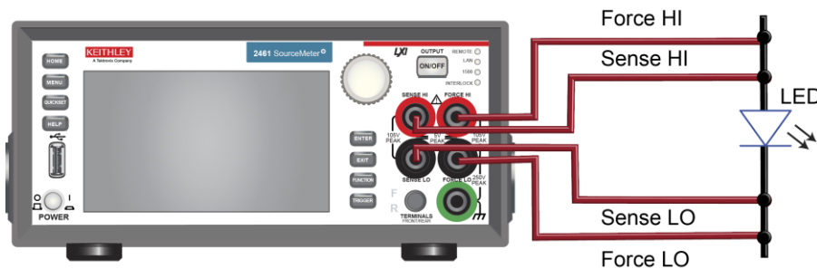
Figure 35: Model 2461 4-wire front-panel connections to an LED
