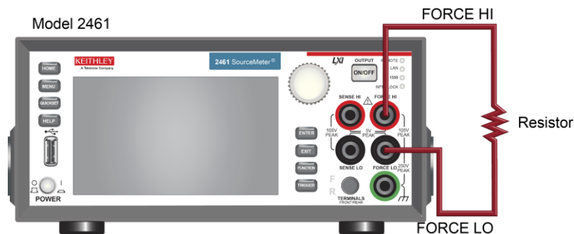
Figure 19: Model 2461 2-wire front-panel connections
