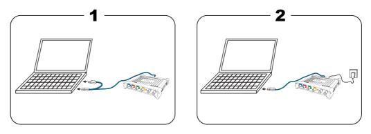
**Note:** If you connect or disconnect the AC adaptor while the oscilloscope is in operation it will restart automatically and any unsaved data will be lost.
