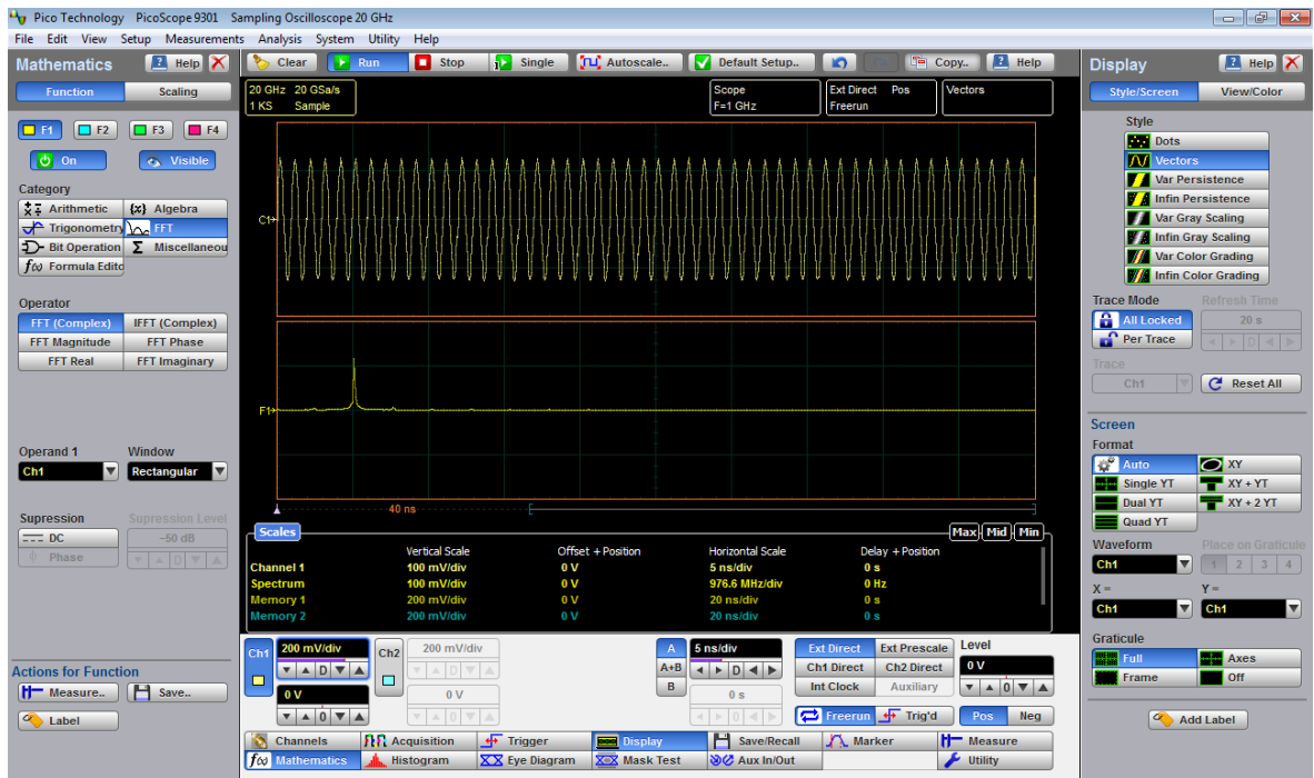
The 1 GHz sine-wave signal shown in both the Time Domain and the Frequency Domain
