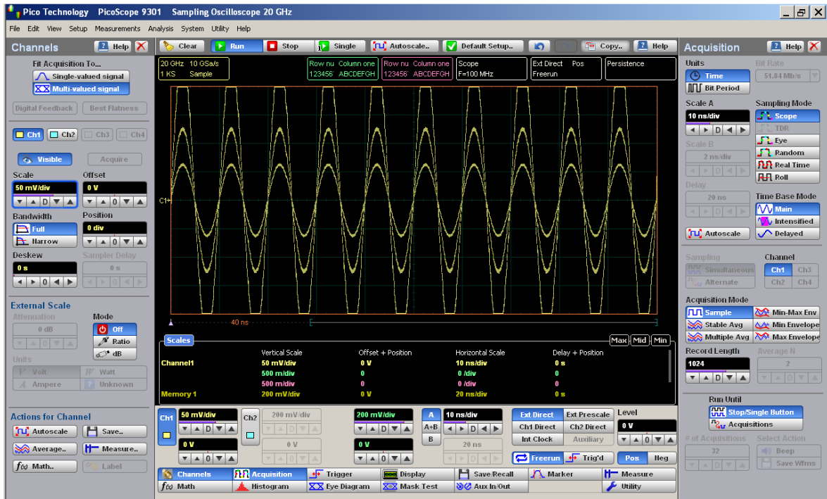
Vertical scaling of a waveform
