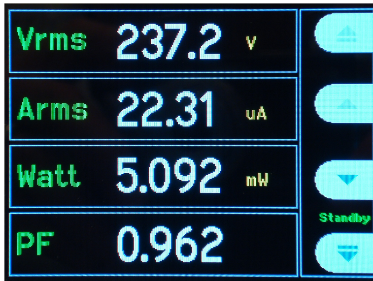
Figure 19: PA1000 measuring 5 mW in front-panel standby mode
