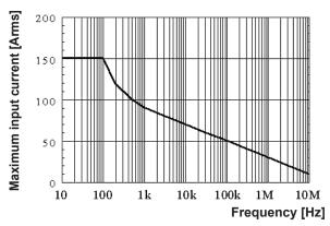
Figure 2 Derating According to Frequency
