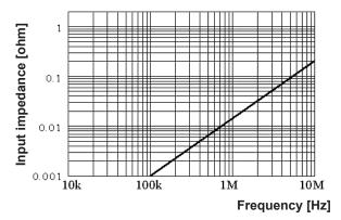
Figure 3 Insertion Impedance (Typical Characteristics)
