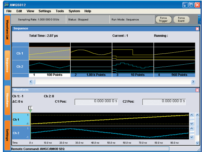
Figure 32. The Graphic editor and Sequence editor are combined for flexible waveform creation.
