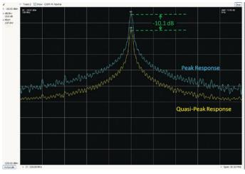
Figure 8. The effect of peak and quasi-peak detection on a signal with an 8 us pulse width and 10 ms repetition rate. The quasi-peak value is 10.1 dB lower than the peak value.
