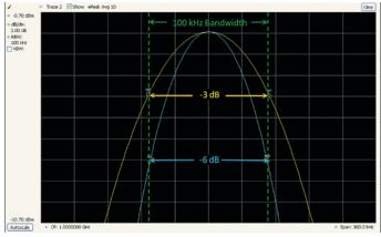
Figure 3. Spectrum Analyzer with selectable -3 dB (RBW) and -6 dB filter definitions, 1 dB/division.
