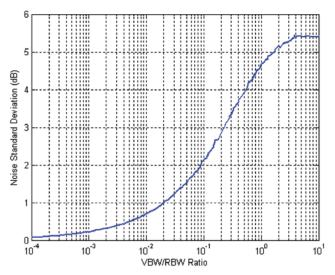
Figure 9. Effect of VBW/RBW ratio on standard deviation of random noise signal. When VBW ≥ 3 times the resolution bandwidth, there is no practical effect on signal deviation from the VBW.
