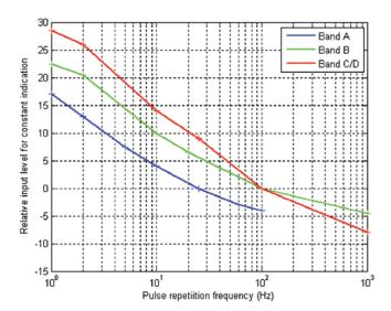
Figure 7. Pulse response curve with a Quasi-peak detector.
