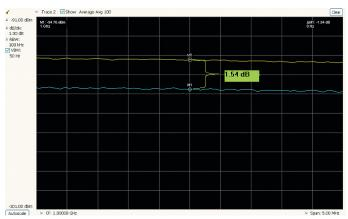
Figure 4. Random noise measured with 100 kHz filters. -3 dB, 100 kHz response in yellow, -6 dB, 100 kHz response in blue. The power difference is 1.54 dB, in close agreement with the theoretical value.
