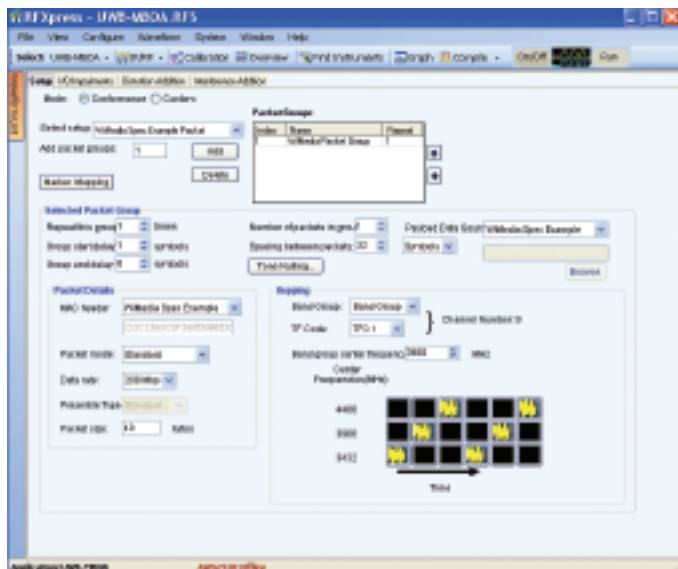
Figure 7. UWB-WiMedia signal generation in RFXpress conformance mode.
