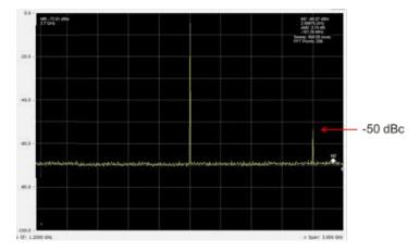
The Tektronix AWG70000 Series centered at 1.2 GHz IF.
