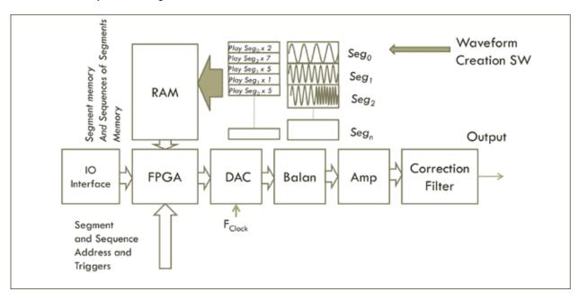
The Tektronix RFXpress® software is used to generate various RF waveforms that are loaded into the instrument through an I/O interface such as LAN, or PCIe. In some cases such as the Tektronix AWG70000 the waveform generation software is native to the instrument, in other cases a separate PC software program is used such as MATLAB®.
