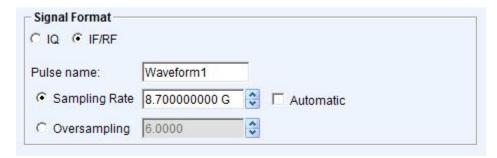
Certain combinations of sample rates, waveform frequency and length will result in sub-optimal SFDR. If the sample rate changes, the time to waveform play out will change as well, so when creating waveforms it is important to keep this sample rate fixed. However if that sample rate causes a worse case SFDR as shown in the table below, then a more optimal sample rate must be chosen and the strobe timing adjusted to keep the system timing accurate.
