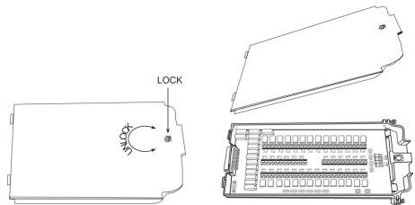
3. Using a small flat-blade screwdriver, loosen terminal screws and install wires as needed. Channel designations for the screw terminals are shown in the following figure.
