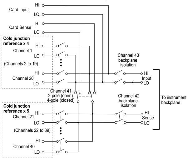
Channel 41 (2W/4W Configuration), Channel 42 (Sense Isolation), and Channel 43 (Input Isolation) are normally automatically configured by the DAQ6510.
