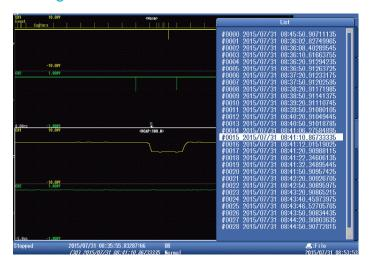
Dual Capture produces a List of capture events when the high-speed sampling was triggered.
