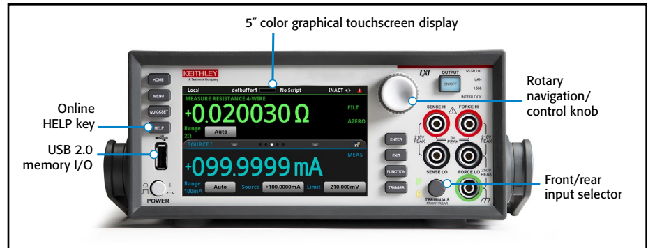
Model 2450-EC front panel with high resolution, capacitive touchscreen.
