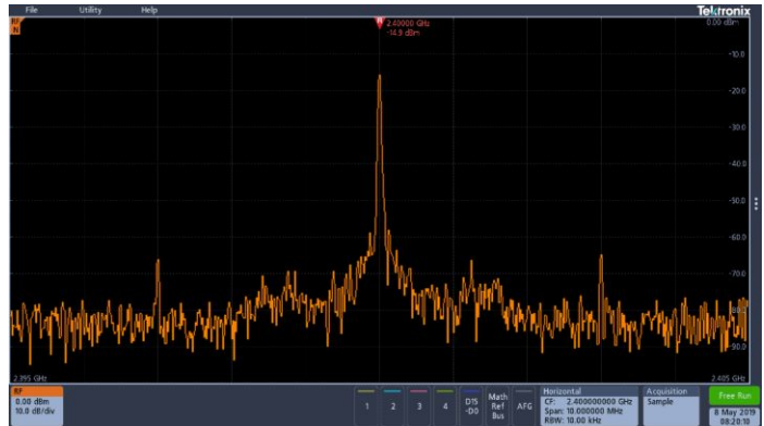
3 Series MDO frequency domain display.
