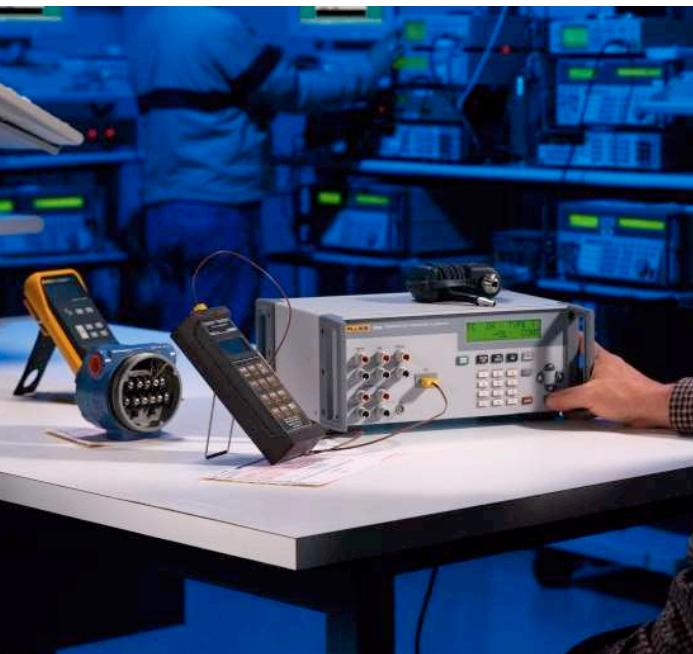
The Fluke 525B Temperature/Pressure Calibrator gives you a workhorse combination of high accuracy and broad functionality for temperature and pressure instrument calibration. Compact and economical, the 525B has an interface for automated calibration, providing wide workload coverage in instrument shops and calibration labs, as well as in ATE applications.
