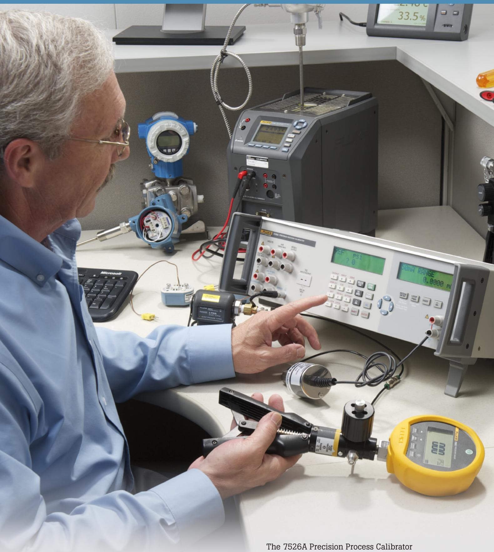
The 7526A Precision Process Calibrator calibrates a wide range of pressure gauges, temperature transmitters, digital process simulators, multimeters and more.
