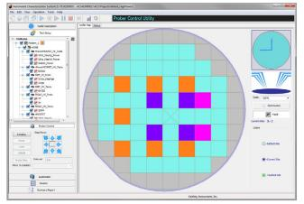
Interactive probe station control speeds and simplifies test development and debugging by combining interactive testing with manual probe station control.
