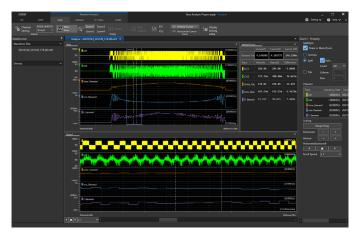
Figure 6. Cursor measurement of power data and waveform data
