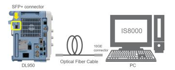
Figure 2. Connection between DL950 and PC
