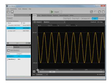
The Tektronix AWG5200 series features a digital complex modulator and multi-rate interpolation. With this internal IQ modulation feature, you remove the IQ mismatches that are attributed to external modulators and mixers. Also with this modulator, there is no in-band carrier feed-through, and there are no images. With its built in interpolators, it also affords the ability to create waveforms most efficiently reducing waveform size and compilation times as well as extending playback time.
