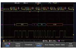
GDS-2000E, MSO-2000E, and MDO-2000E series can trigger and decode the Serial interfaces, SPI, UART, I2C, CAN and LIN. Each input can be displayed as binary, hexadecimal or ASCII. These can be displayed not only as a serial bus signal but also as the Event table.
