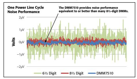
Comparison of the Model DMM7510's 1V DC noise performance with that of typical 61/2- and 8½-digit multimeters. All data was taken at 1 NPLC with a low thermal short applied to the input.
