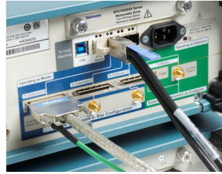
UltraSync connection on instrument with Master role
